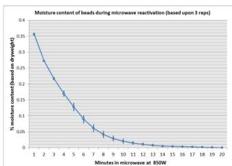
A microwave can be an excellent device for regenerating small quantities of drying beads. A microwave is available on a worldwide scale and is more and more a standard appliance in most kitchens. A few precautions have to be made, because in the worst case you could heat up your beads to a temperature higher than 500°C and even melt the beads these precautions are:
