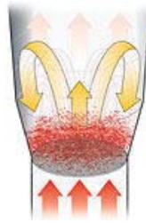
Working principle of fluidized bed
