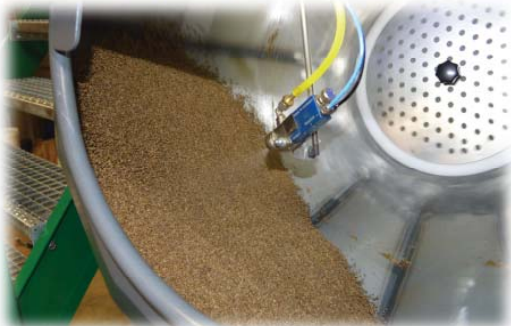
ICD in coating position
