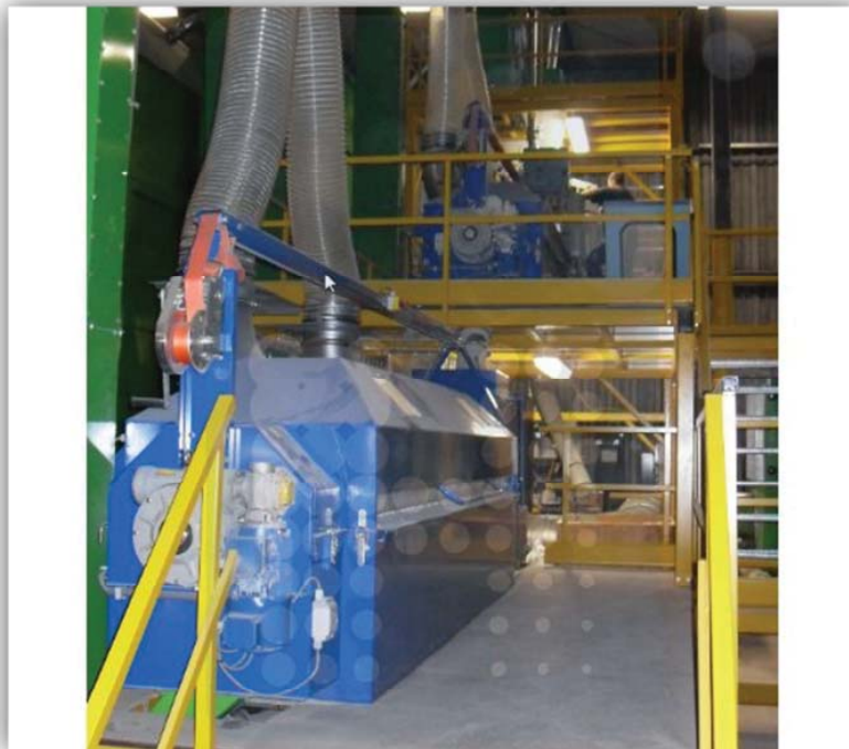
Double RFBD600-19 Dryer for grasscoat 1:1 1250kg/h
